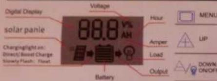
Menu key: switch parameter display interface, long press 3s-5s to enter or exit parameter setting.
